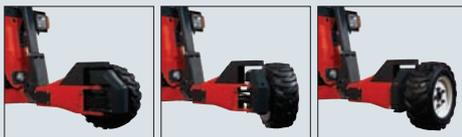
The **4-way** model can also carry loads sideways, ideal when delivering long loads into tight access areas or through narrow passageways.
